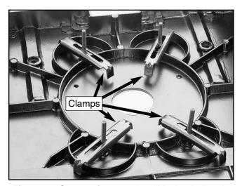
**Figure 8.** Clamps for securing "**Method 2**" style routers to the main table.
